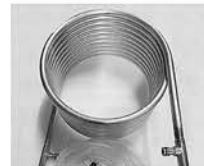
(c) Heat Exchanger
