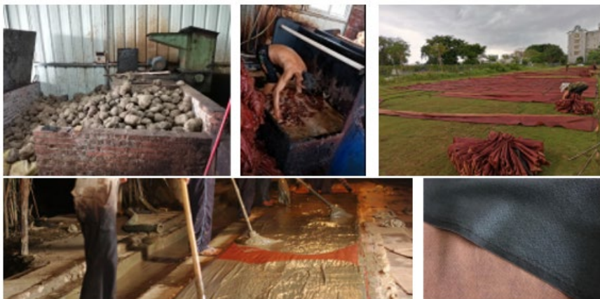
Figure 1 Brief Steps of Dyeing and Finishing of Gambiered Guangdong Silk Source: Author
